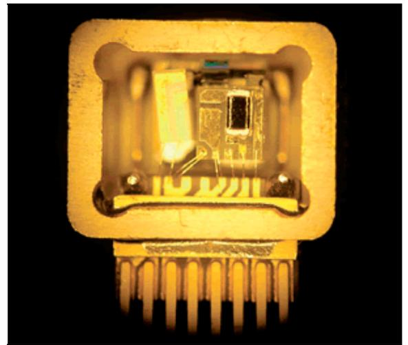
Figure 1. The 3D nature of optoelectronic packages makes these systems different from electronics, which are predominantly 2D.
